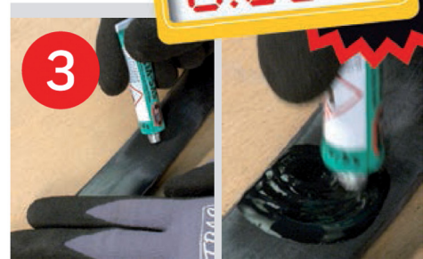
3 Apply the SVS Vulcanizing fluid even and thin on the clean buffed repair area
