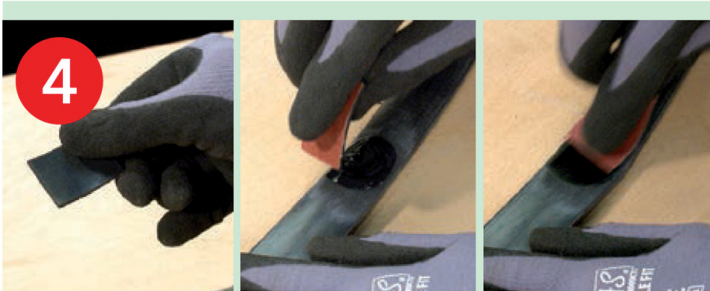
4 ✓ Slightly spread the SVS Vulcanizing fluid with the rubber edge of the special-combi-pad 5 x times crosswise until the SVS is silky gloss.
